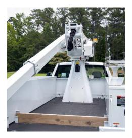
SINGLE HANDED ERGONOMIC UPPER CONTROLLER CAN BE MOVED BETWEEN TWO POSITIONS FOR OPTIMAL OPERATOR COMFORT
