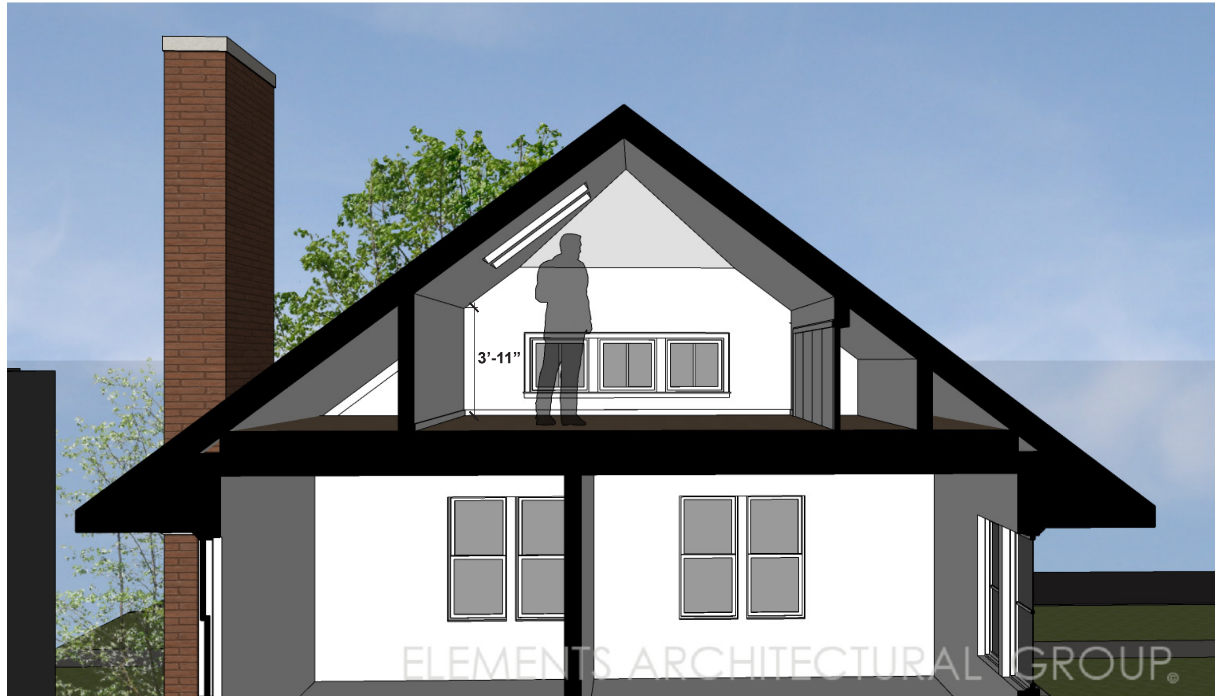
SECTION THROUGH EXISTING HISTORIC ROOF. DESIGN INTENT IS FOR THE HISTORIC CLIPPED GABLE RIDGE AND ROOF TO REMAIN, LOW CEILING REQUIRES DORMERING.
