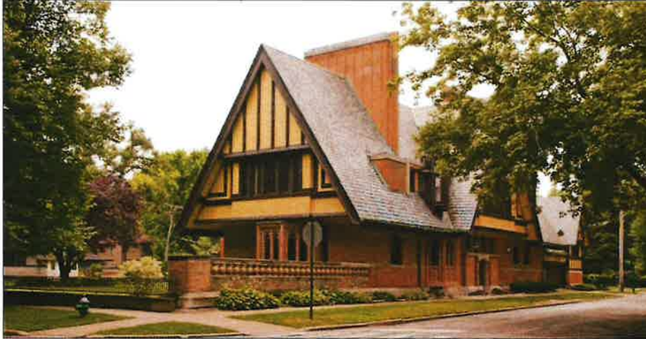
A roof and its associated features, including form, materials, chimneys, dormers, and overhanging eaves, can be key elements in a building's style.
