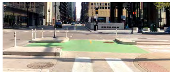
Example of a protected intersection.
