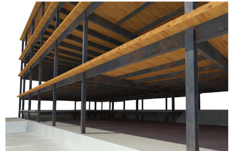
Steel Frame with Timber Floor
