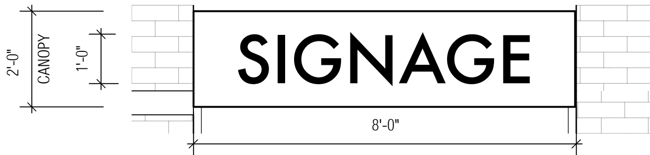
Residential Entry Signage Elevation Scale: 1/2" = 1'-0"
