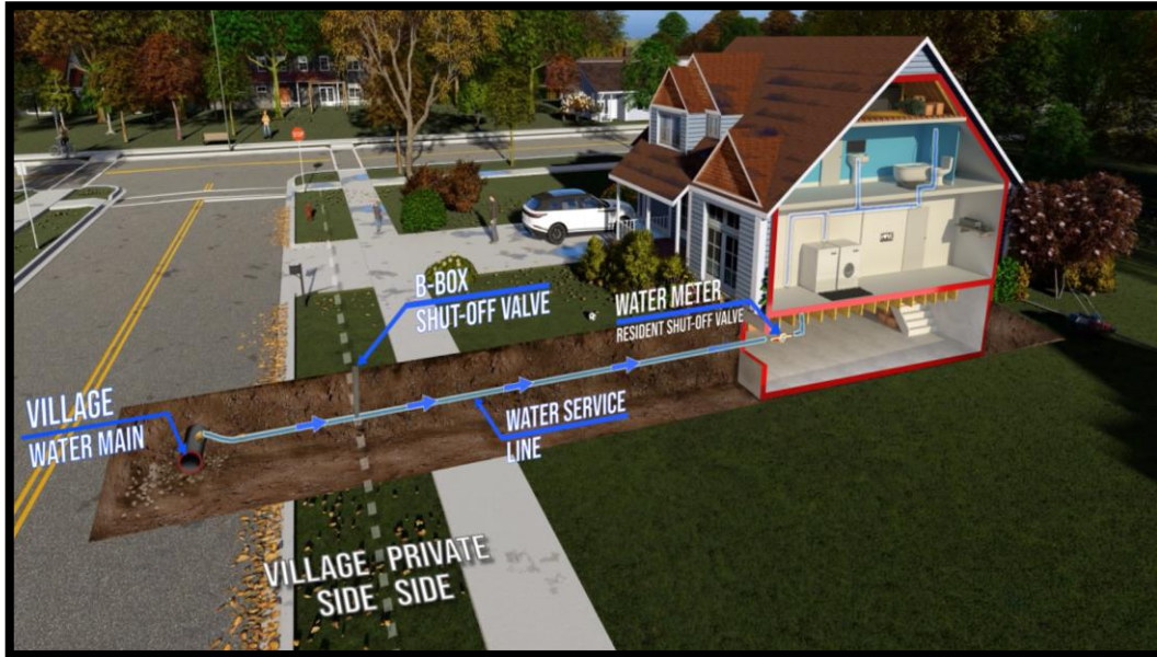
Figure 2: Water Service Line Ownership
