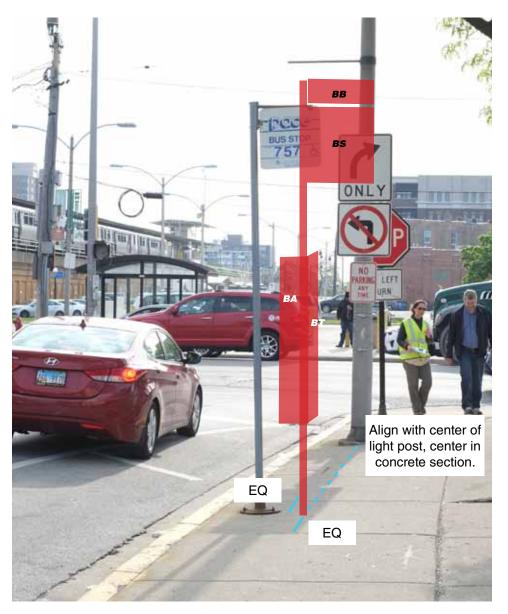
New sign panels, cabinets, sign post, and base replace existing sign post and base.
