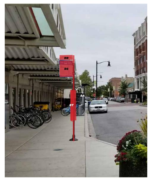
New sign panels, cabinets, and sign post replace existing. Existing base to remain.
