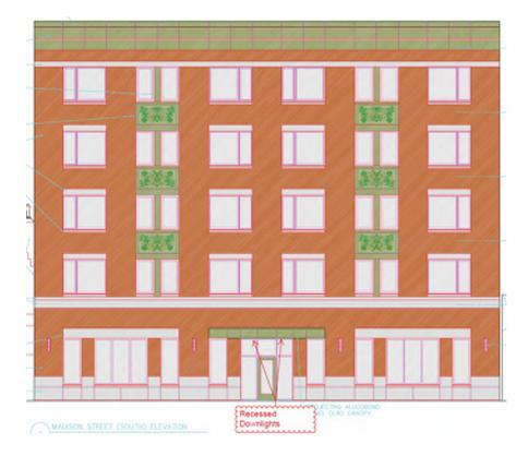
The Illuminating Engineering Society recommends light levels within the range of 2-4 foot-candles at the main entrance of a building. These recommendations take into account that a light loss factor (LLF) is typically used when calculating light levels. Light loss factors address the fact that over time light output is decreased from all lighting fixtures.
