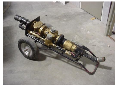
Calibrated portable test meter.
