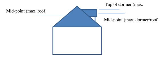
If the mid-point of the roof is at its maximum height, then the top (ridge) any dormer could not be higher than the mid-point of the roof. If the dormer height is measured at its mid-point, it would be closer to that of the building mid-point – depending on the size / location of the dormer. Is this the best way to measure the height of a dormer?
